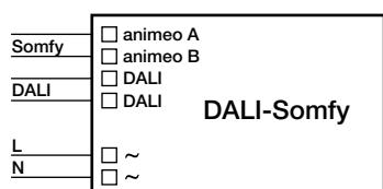
The polarity (A, B) between the DALI-Somfy module and the Somfy motor controller must be observed.
