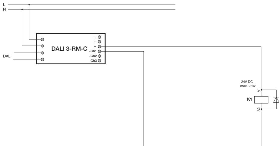
Outputs Ch1 and Ch3 may not be short-circuited. The entire output may flow via one output.
