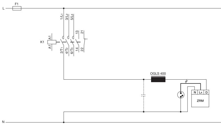
Please check the inrush currents of the switched loads. Electronic control gear may have very high inrush currents. Check with the contactor manufacturer.
