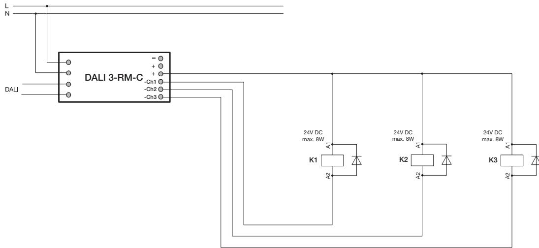
The contactors must be equipped with an appropriate threshold diode. Operation without a threshold diode is not permitted.
