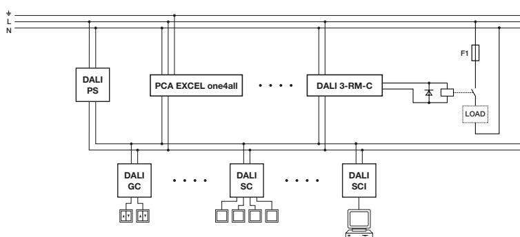
**Circuit diagram for three contactors with a maximum power of 8 W**
