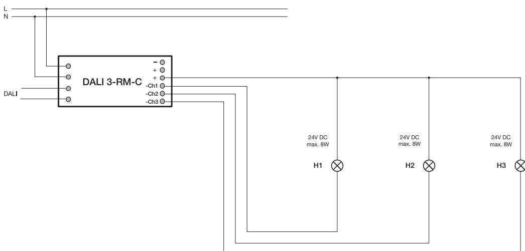
Signal lamps can be connected directly. The controller is designed for a maximum load of 25 W. This load can be split among the three channels. The loads may be distributed asymmetrically.
